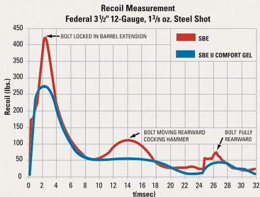
BENELLI ENGINEERS developed specialized machinery to measure and graph recoil. Here a Benelli Super Black Eagle is plotted along with an SBE II with ComforTech™. A dramatic reduction with ComforTech™ can be seen in all three peaks of recoil – firing, bolt cocking the hammer and the end of bolt travel.
