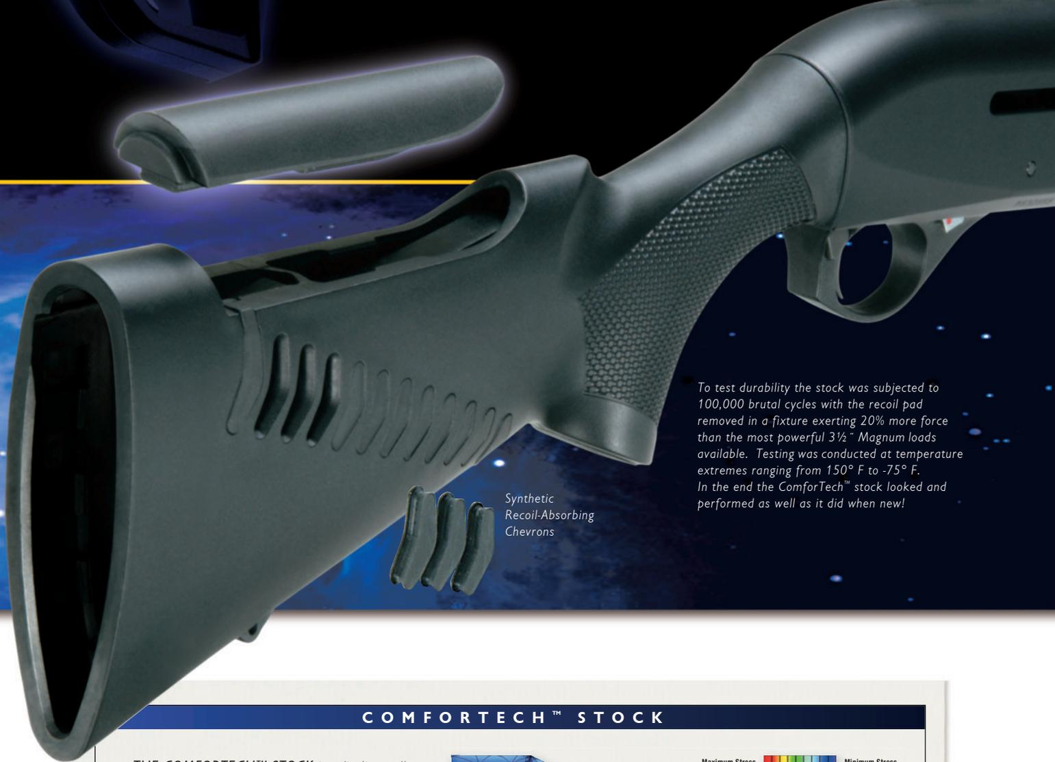
To test durability the stock was subjected to 100,000 brutal cycles with the recoil pad removed in a fixture exerting 20% more force than the most powerful 3 1/2" Magnum loads available. Testing was conducted at temperature extremes ranging from 150° F to -75° F. In the end the ComforTech™ stock looked and performed as well as it did when new!
