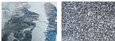
Untreated      Cryogenically Treated
