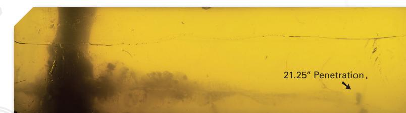
Bone in gelatin shot with 165-grain .30-06 Springfield Trophy Copper (P3006TC2) from a Kimber 84L at 100 yards. All Federal Premium® bullets are tested in ballistic gelatin to ensure proper performance.
