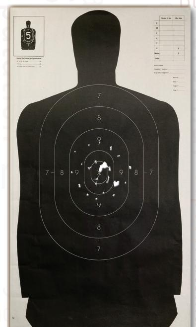
Target shot with 12-ga 2-3/4" 4 Buck, 34 pellets (PD156 4B) with improved cylinder choke in a Benelli Super Black Eagle II at 5 yards.
