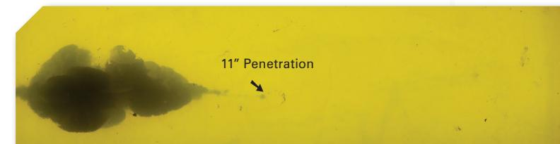
Gelatin shot with 55-grain .223 Rem. Nosler Ballistic Tip Varmint (P223F) from an AR-15, 16-inch barrel, 1:9" twist at 100 yards. Ballistic Tip Varmint rounds are incredibly accurate, rapid expanding and dump energy in game with minimum penetration—ideal for varmint hunters.
