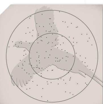
PF154FS 4 puts over 75% of its pattern in a 30-inch circle at 40 yards with a modified choke.
