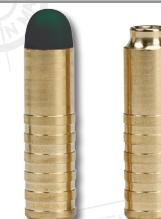
The Woodleigh® Hydro Solid's polymer cap disintegrates on impact, exposing a concave nose and flared pressure ring. It creates a larger wound cavity than traditional solids.
