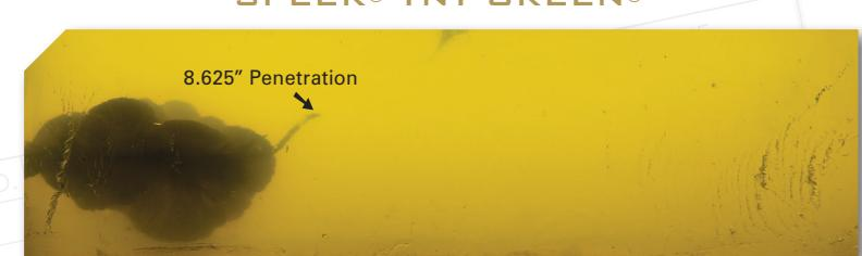
Gelatin shot with 43-grain .223 Rem. Speer TNT Green (P223R) from an AR-15, 16-inch barrel, 1:9" twist at 100 yards. TNT Green loads explode on impact—creating only an entrance wound and transferring all of their energy inside the target.
