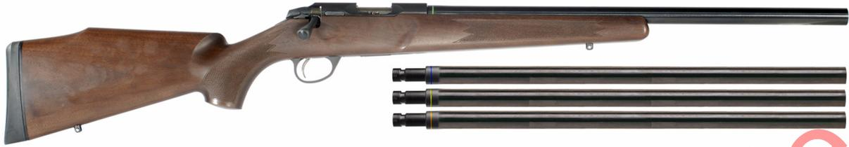
SAKO QUAD VARMINT rimfire rifle based on P04R action. The gun can be easily converted by customer to calibers 22 LR, 17 Mach 2, 22 WMR or 17 HMR by changing only the barrel and the magazine, if necessary (Pat. pend.). Barrel changing tool included with each rifle.
