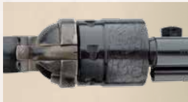
The 1860 Army Conversion revolver frames had to be fitted with spacers in order to function properly and safely with the shortened cartridge conversion cylinders.
