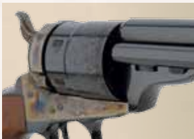
The conversion revolvers were also fitted with ejector rods, a necessity for removing fired casings from the cylinder.
